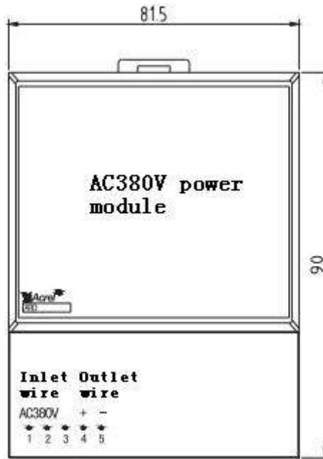
Figure 9 Outline dimensions of AC380 power module
